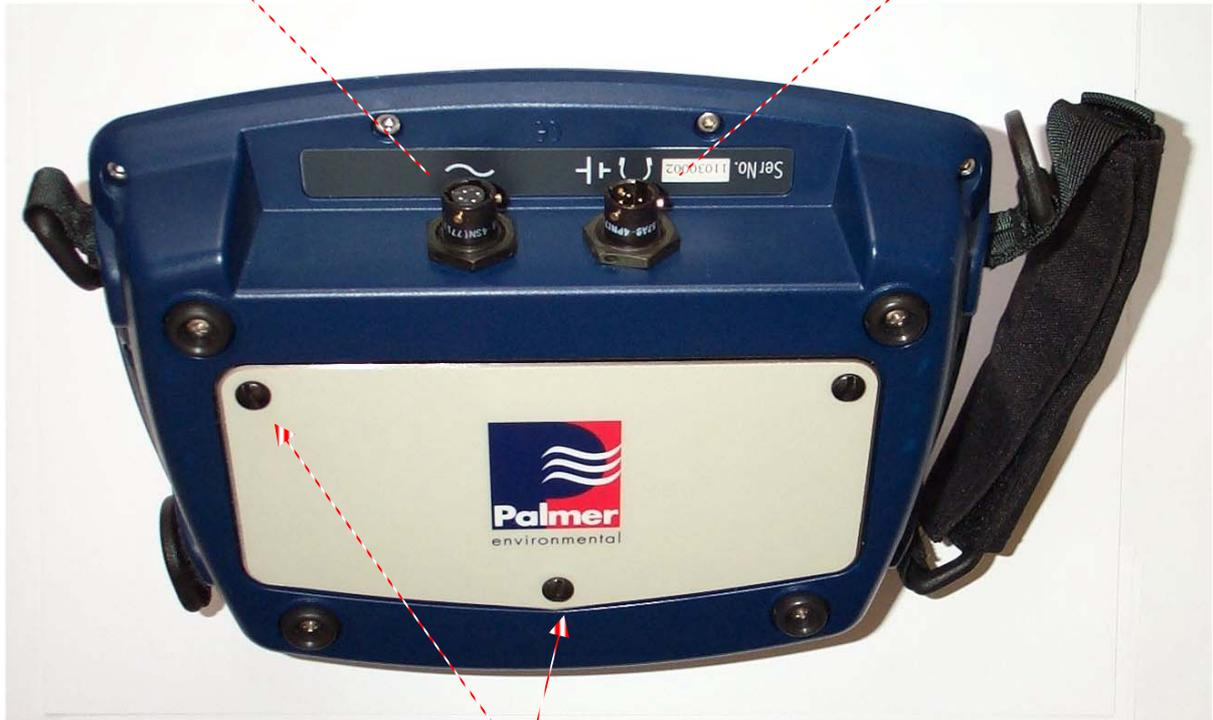
Three retaining screws
